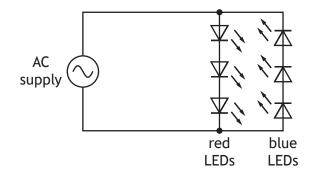
The red LEDs and blue LEDs each flash twice per second.
