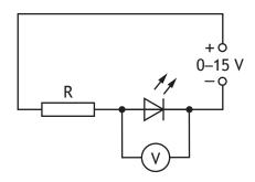
The student adjusts the voltage output of the variable power supply until they see the LED start to emit light.
