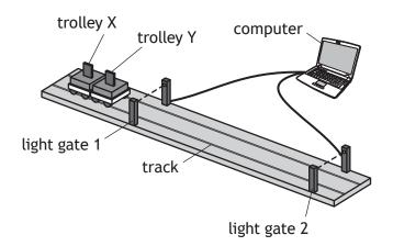
The trolleys X and Y are moving together to the right at 0.40 m s<sup>-1</sup>.
