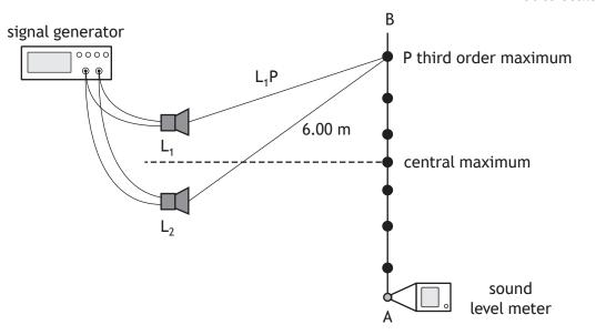
A sound level meter is moved from A to B, and a series of maxima are detected.
