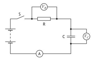
The capacitor is initially uncharged. Switch S is closed.
