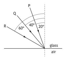
The refractive index of the glass for this light is 1.50. Which of these rays pass from the glass into the air at this boundary?
