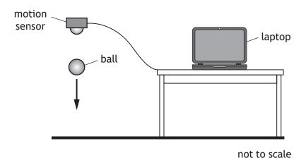
The ball is released from rest below the sensor.
