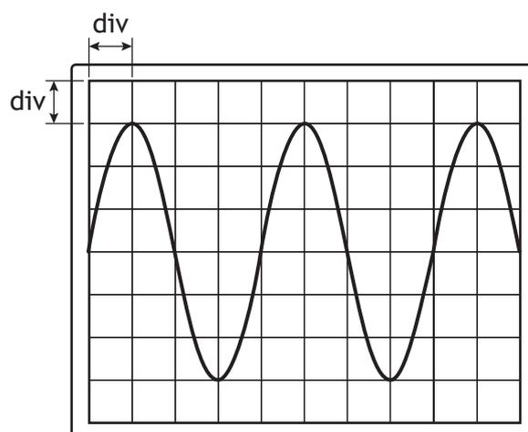
The Y-gain setting on the oscilloscope is  $1.0\text{ V/div}$ .
