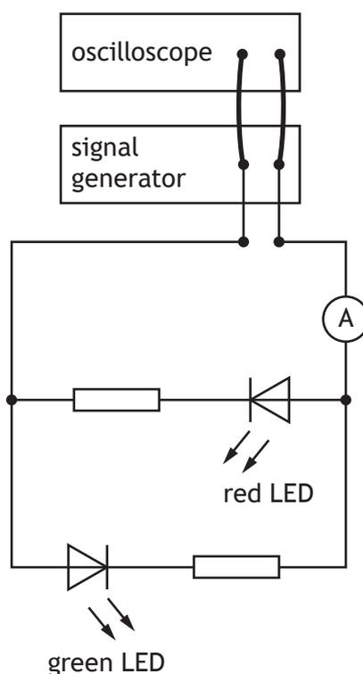
The output of the signal generator is displayed on the oscilloscope.
