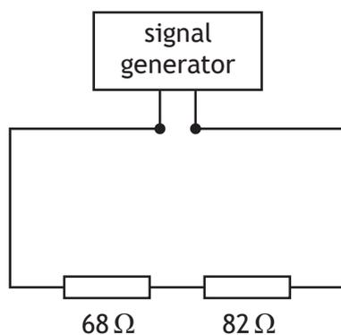
Determine the r.m.s. voltage across the  $82\ \Omega$  resistor.
