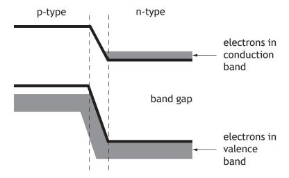
LEDs emit light when electrons fall from the conduction band into the valence band of the p-type semiconductor.
