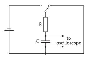
Which pair of graphs shows how the potential difference V across the capacitor varies with time t during charging and discharging?
